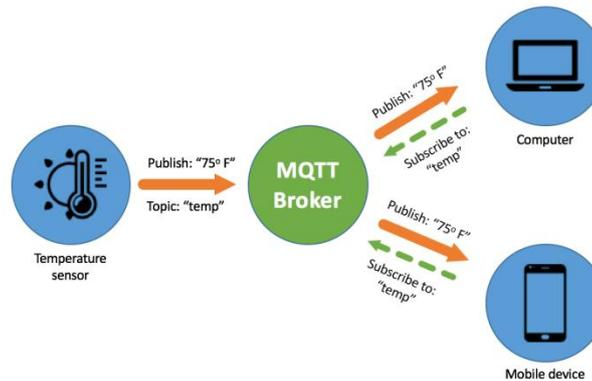
Figure.1. Model of communication protocol
